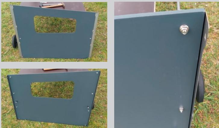
Place the sheet metal fittings on the right side wall from the outside and place the **number 10 screws** and **number 3 nuts**.
